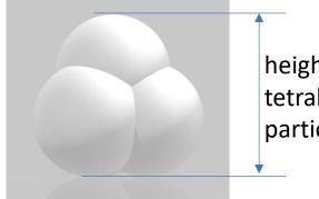
height for tetrahedral particle Each clump is made up of four spheres that have the same diameter of 6.2020mm. The four sphere centers are placed at the vertices of a tetrahedron and so the particles can be called tetrahedral particles. The clumps were generated by a 3D printer. The circumsphere that acts as an envelope to the clump is 10 mm (1 cm) in diameter.
